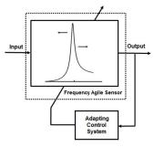
Fig. 5 – Diagram overview of the feedback control system used to achieve dynamic frequency adaptation.
