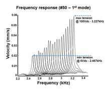
Fig. 4 – Frequency response of the Kapton membrane while providing different tensions. Driving voltage vs natural frequency response.
