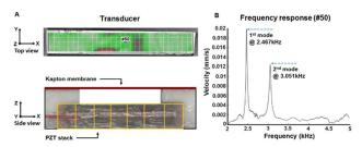
Fig. 3 – (A) Acoustic transducer built with a Kapton membrane and a PZT stack. (B) Frequency response of the transducer showing 2 resonance modes.
