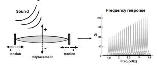
Fig. 2 – A fixed-fixed beam structure as a simple system to model the behaviour of the tympanic membrane of moths. Frequency response is changed by increasing tension.
