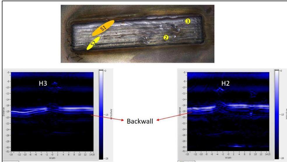
FIGURE 11. TFM (5 MHz) to detect H2 and H3
